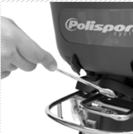
**EN.** Screw nut M8 (N) onto bolt M8x25 (M). Tighten the nut using a no. 13 open-ended spanner. Make sure that the nut is properly tightened and that the luggage carrier fixing base (I) is properly attached to the baby seat.
